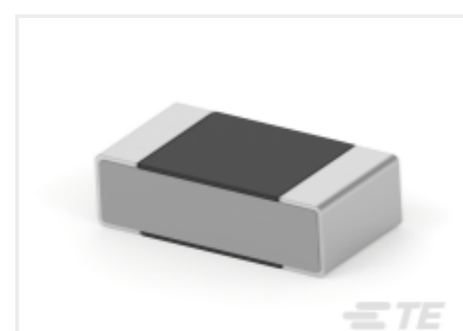
TE 产品编号5-1879207-8 RN 0603 392K 0.1% 10PPM 5K RL
