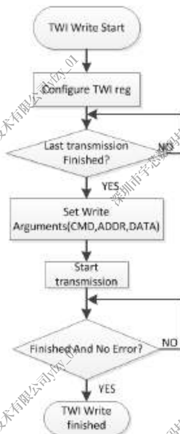
Figure 12-5. TWI Write Flow
